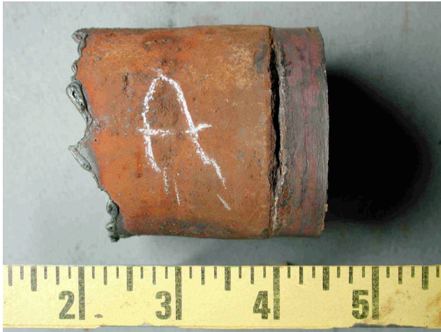
Figure 1. End of boiler tube showing typical features of failure: groove and crack adjacent to band where tube was rolled into tubesheet.
